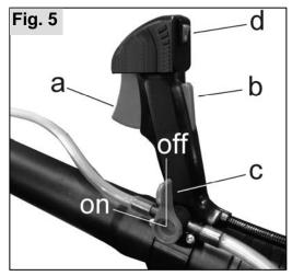
To release the throttle control (a):
