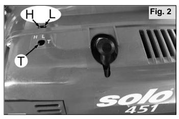
The carburettor has 3 adjusting screws (Fig. 1 - 5):
