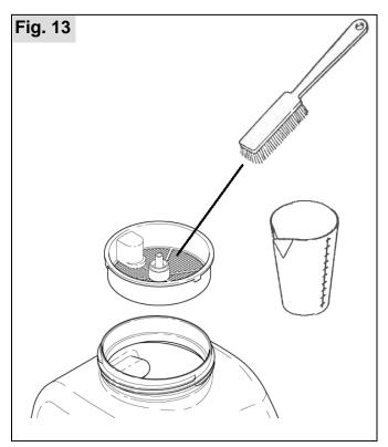
Occasionally clean the strainer inside the filler neck, the strainer in the accessory set and all parts in contact with the medium, with water and a soft brush.
