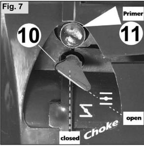
Close choke with choke lever (10).
