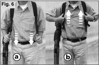
Place the mistblower on the back and connect to quick couplings on either side.
