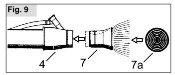
When spraying plants and trees we recommend fixing the wide-range nozzle (7) onto the red standard nozzle (4). This ensures that a large area can be sprayed at one time. Push the wide-range nozzle onto the standard nozzle, until the bead engages.
